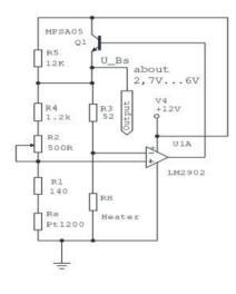
Both elements (Heater RH and sensor RS) can be switched in a bridge. The resistors R1,R2 and R3 are to dimensionate rightly to balance the bridge between RS and RH at a selectable temperature difference ( $\Delta$ T). This is the condition to which the voltage fitting to the bridge is controlled.
