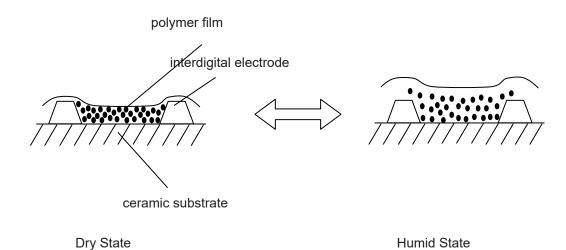
The dew sensitive polymer film in which conductive particles are dispersed in polymer which expands by water shows a low electric resistance by the contact of carbon under the conditions of dry atmoshere.
