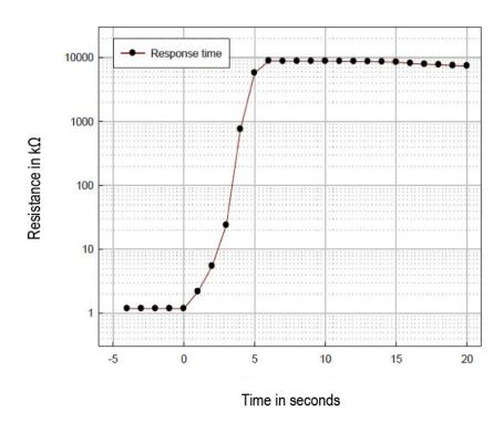
Resistance characteristics at dipping water (Test condition: 25 °C Dew condition)
