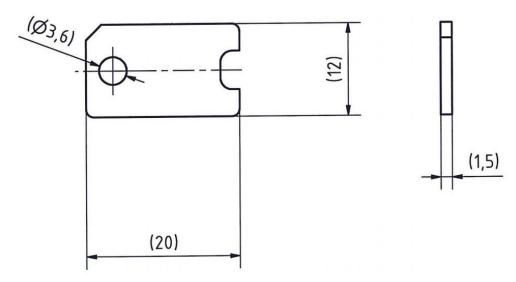
The hole distance from the top to the edge is 2 mm. The hole is made exactly in the middle.
