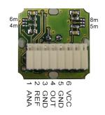
There are four soldered joints on the back side of the module. By closing (over-soldering) one of the jumpers, the sensitivity of the module can be reduced.
