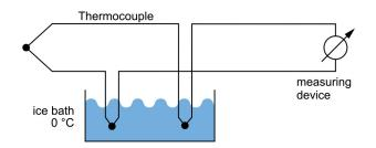
Usually the temperature connection point is determined by means of an absolute measurement method, for example with a PT 1000. Then, it is possible to mathematically compensate the temperature of the connection point.
