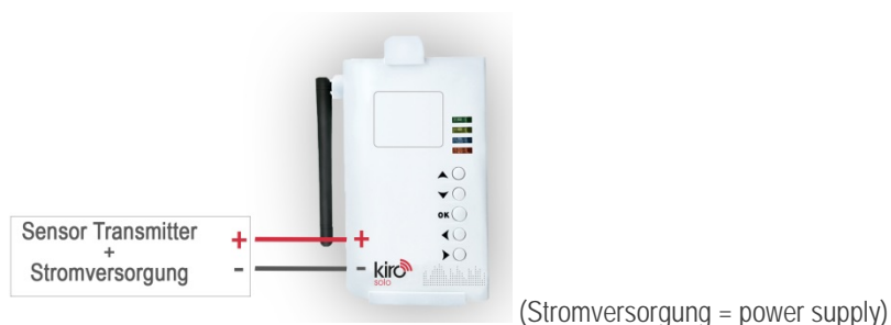
Figure 13: Connect positive signal output of the kiro solo transmitter to pin 3 [+] of the universal kiro solo and connect negative signal of transmitter to pin 4 [-] of the universal kiro solo
