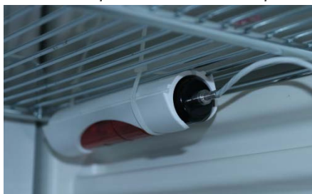
Figure 10: Under the rack field mounted probe with glycol vial
