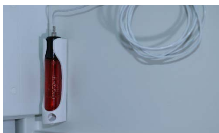
Figure 11: At side wall mounted probe with glycol vial
