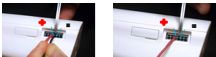
Figure 17: Pressing down into the top rectangular opening, inserting the wire, removing the tool.
