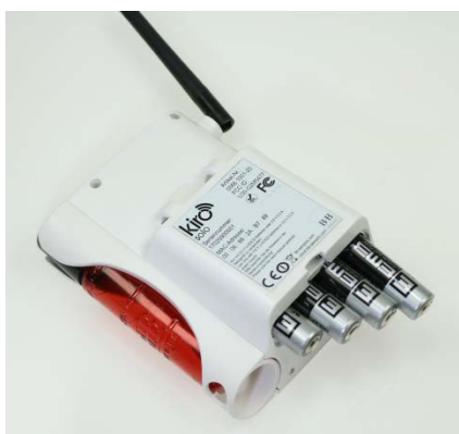
Figure 3: Insertion of batteries
